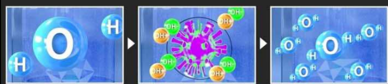
Creation of hydroxyl (OH·) through electrolysis of water molecules
